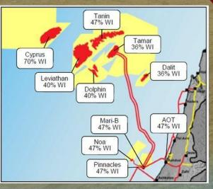
Drill 8 wells to ~ 5000 m Install subsea development @ 1700 m Install 150 km of dual 16" pipelines Build and transport Tamar platform Install Tamar platform near Mari-B
